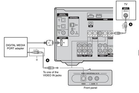
\* The type of connector varies depending on the DIGITAL MEDIA PORT adapter. For details, refer to the operating instructions supplied with the DIGITAL MEDIA PORT adapter.
